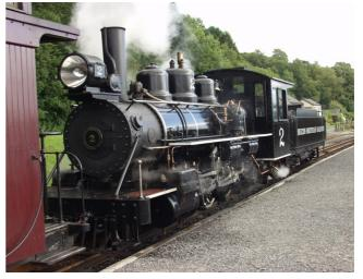
carriages drawn by a 4-6-2, 47 ton American Narrow Gauge steam locomotive "No 2" (2 foot gauge, made by the Baldwin Company of Philadelphia in 1930) complete with bell and two-tone whistle steaming through part of the Brecon Beacons National Park alongside the large Taf Fechan reservoir. This experience was topped with a cornet of Sidoli's Ice Cream on the return journey!
